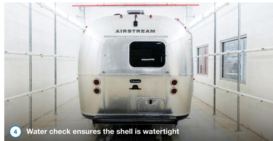
4 Water check ensures the shell is watertight
